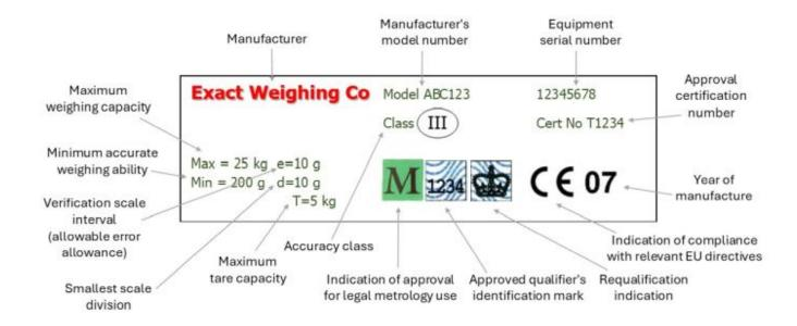
Newer equipment may also have some of the required markings indicated on the equipment's display screen rather than permanently displayed on the equipment body.
